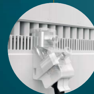
Conductor connection terminal with integrated cover for copper and aluminium conductors. It is suitable for 1 round or 1 sectored conductor up to 240 mm².
